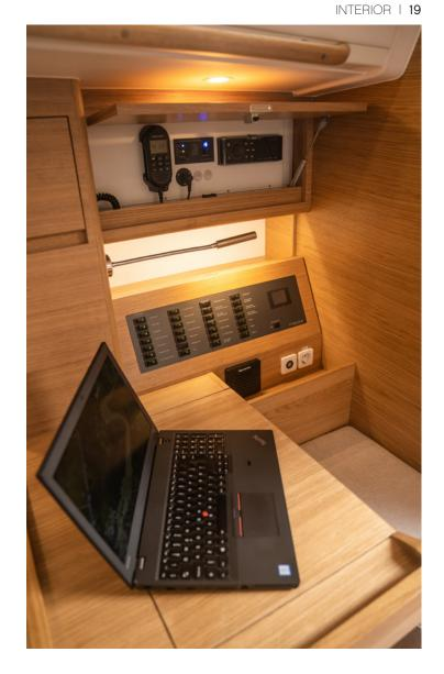
Above: The nav station is the X46's communication centre as well as the main hub for the yacht's electrical systems.
