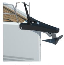
Optional carbon bowsprit in clear coat finish, with integrated anchor fitting.
