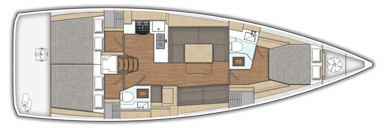
Standard Layout - 3 double cabins, 2 heads, aft cabin standard
